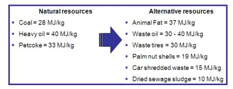
The use of waste into the cement industry does not only replace traditional fuel but can also recover valuable raw material. For example the foundry sand which is a waste of the foundry industry can easily replace the Silicates required in the cement industry. Many other examples exist and we could strive to a sort of industry ecosystem where the wastes of some industries become alternative resources for others.
